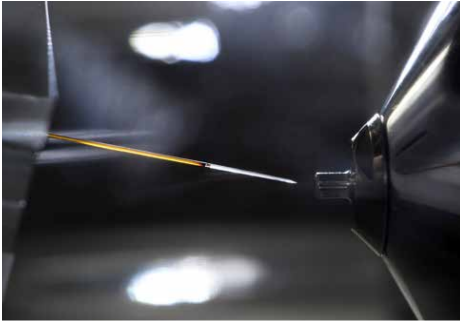
This precision device, which couples liquid chromatography and mass spectrometry, is used to identify and quantify proteins.
