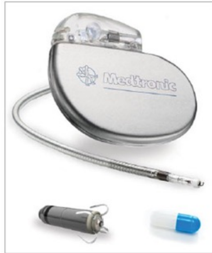
Figure 2 Comparison of the size of traditional and next generation pacemakers in relation to a capsule
